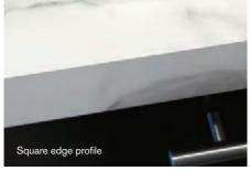
**Square edge** is made by clashing the benchtop edge with a piece of the same laminate to create a true square edge. A traditional Formica<sup>®</sup> laminate look, a dark line will be visible on lighter colours.
