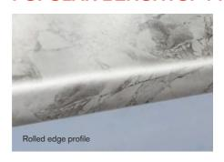
Rolled edge. Formica® 180fx® laminate can be rolled to a minimum radius of 8mm. A rolled edge provides a clean, consistent look with no joins, is cost effective, and extremely hardwearing with very good chip and impact resistance. It is also ideal for environments where pointed edges need to be avoided or impact with the body might occur.
